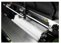
The cleaning agent spraying device is able to accord to PCB size adjusting the filling amount and area automatically.
