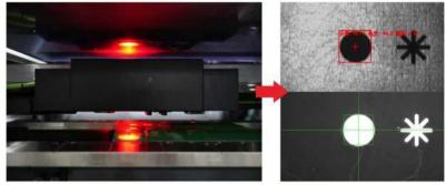
Coaxial image CCD up and down double, adaptive Lighting automatic adjustment; Camera Automatic Recognition of Various MARK Point Graphics.
