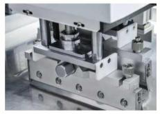
Squeegee adaptive floating head\* front and rear squeegee Lift controlled by Independent motor, printing with constant pressure.
